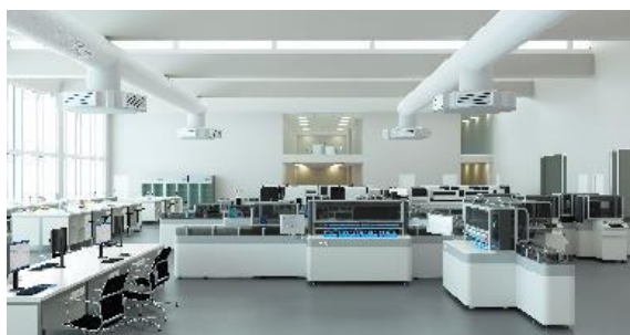
Inpeco FlexLab™ X latest-generation Total Laboratory Automation system.
