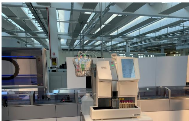
Tosoh's HLC-723™GR01 HbA1c analyser connected into Inpeco's FlexLab™ X Total Laboratory Automation system.
