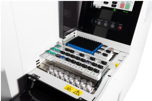
AIA<sup>®</sup>-CL300 reagent cups and samples easily placed in the front table
